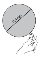
2) Provide the loudspeaker connection cable through the mounting hole in the ceiling. Make sure the used connection cable is sufficiently thick. The required cable thickness depends on its length.
